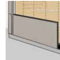
3m pre-finished panels slot into starter track
