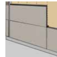
Further panels slot into top of clips and process is repeated....
