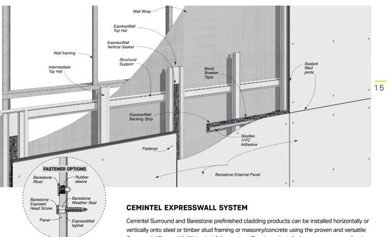
Commercial ExpressWall® top hat fixing system. Panels are installed as a pressure equalised ventilated cavity system which is easy to install and delivers a high weather performance system. Learn more about this system in the Barestone Design and Installation Guides: cemintel.com.au/technical
