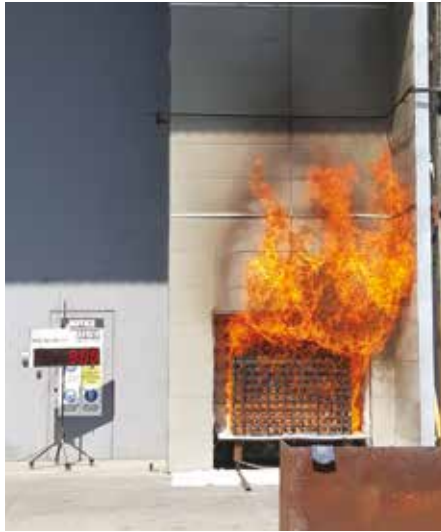
Intensive flames and heat during fire test.
