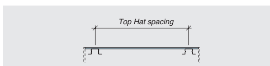
FIGURE 6.07 Panel Fixed to Two Top Hats Only
