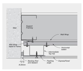
FIGURE 8.16 Vertical Gasket and Fixing Detail for Half-bond Panel Layout
