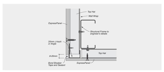
FIGURE 8.30 External Corner – Sealant filled
