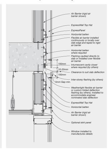
Note: Drawings are interchangeable for timber or steel substrates with the exception of the fasteners.
