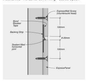
FIGURE 7.19 Vertical Joint – Sealed Option
