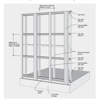
Alternatively ExpressWall framing can be fixed to appropriately designed steel or timber framing. The frame must be designed to support the top hats at the top and bottom of the wall and at cross members within the span of the wall (Refer Fig 4.08).
