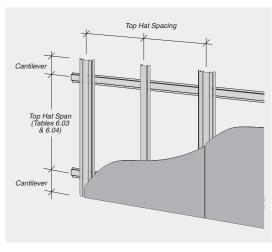
FIGURE 6.05 Double Top Hat Span Installation
