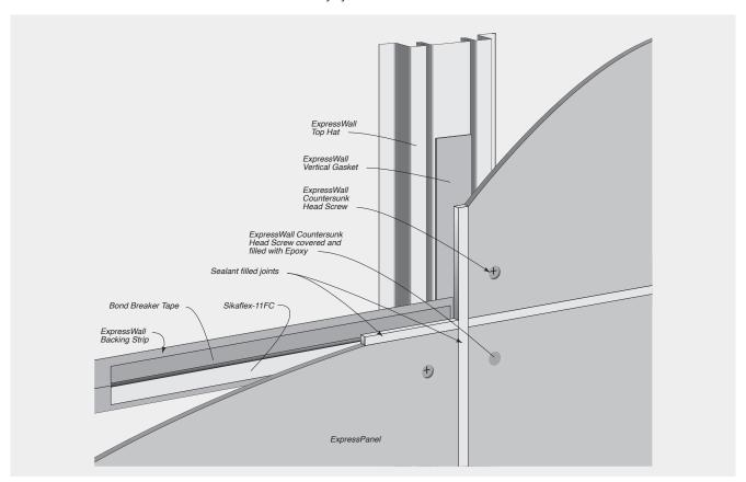
FIGURE 8.23 Backing Strip Preparation
