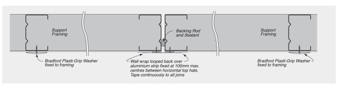
FIGURE 8.42 Vertical Wall Wrap Junction - No Lap Double Washer
