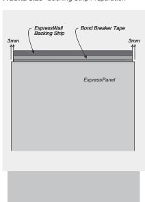
FIGURE 8.24 Horizontal Joint - Sealant filled
