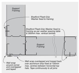
FIGURE 8.34 Internal Corner - Wall Wrap Continuous
