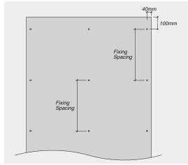
Panels must be fixed in accordance with the tables set out in 'System Engineering' section. This provides fixing Requirements and Maximum Top Hat Spacings for 1200mm wide panels based on 2 top hats or 3 or more top hats.
