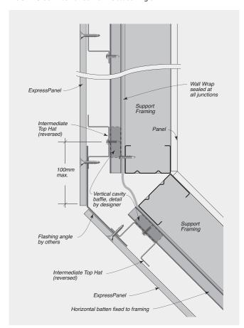
FIGURE 8.10 Internal Corner Detail
