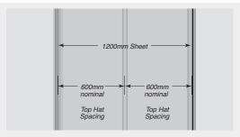
FIGURE 4.02 Horizontal Sheeting Aligned Grid Pattern
