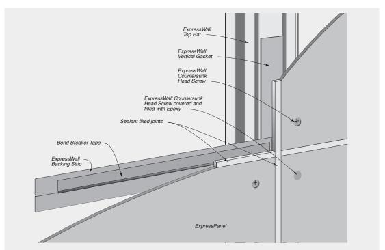
FIGURE 7.15 Horizontal Joint Sealed Side
