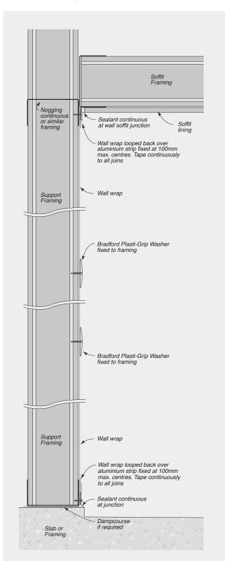
FIGURE 8.38 Wall Wrap Installation at Intermediate Level Junction
