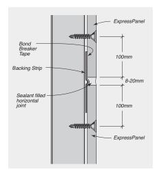
FIGURE 8.25 Vertical Joint - Sealant filled
