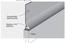
FIGURE 7.10 Sealing Ends of ExpressWall Backing Strip
