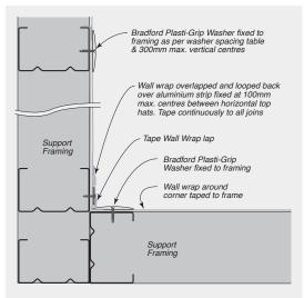
FIGURE 8.36 Abutment to Concrete or Masonry Wall
