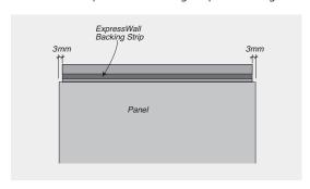
FIGURE 7.09 Horizontal Joint with ExpressWall Backing Strip
