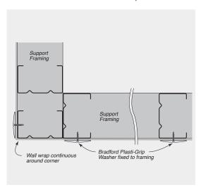
FIGURE 8.33 External Corner - Wall Wrap Overlapped
