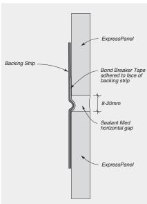
FIGURE 7.17 Backing Strip & Bond Breaker Tape
