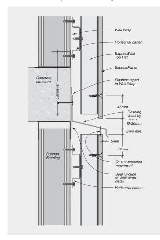
FIGURE 8.14 Inter-Storey Junction with Flashing
