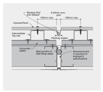
FIGURE 8.13 Inter-Storey Junction with Flashing
