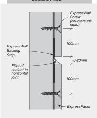
FIGURE 8.03 Horizontal Joint - Angled Backing Strip
