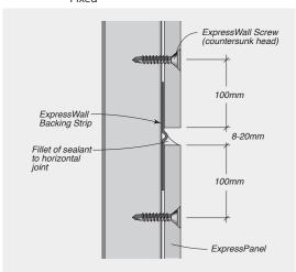
FIGURE 7.13 Countersunk screw head
