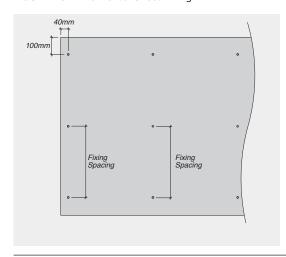
FIGURE 7.02 Vertical Sheet Fixing
