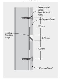
FIGURE 8.04 Vertical Joint - Exposed Head Screw
