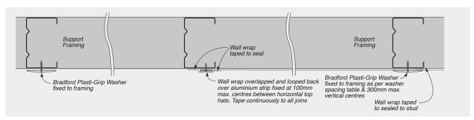
FIGURE 8.41 Vertical Wall Wrap Junction - At Control joint
