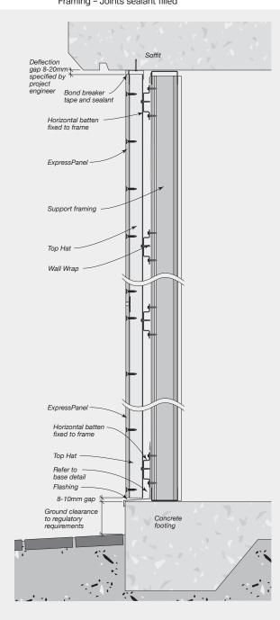
FIGURE 8.27 Eaves/Deflection Head - Sealant filled
