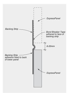
FIGURE 7.16 Horizontal Joint Sealed Side
