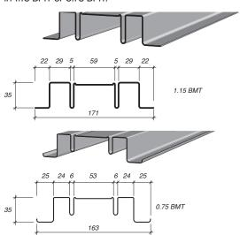
**Intermediate Top Hat** is used to support the panels at intermediate locations in between ExpressWall top hats. The Intermediate top hat is a rolled steel section which is manufactured from galvanised steel (Z275) of 1.15mm BMT.
