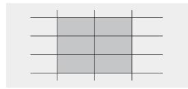
FIGURE 4.03 Vertical Sheeting Aligned Grid Pattern
