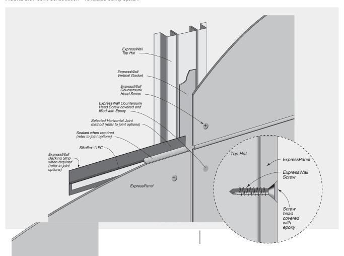
FIGURE 8.02 10mm Horizontal Joint – Sealant Filled
