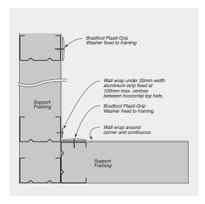
FIGURE 8.35 Internal Corner - Wall Wrap Overlapped
