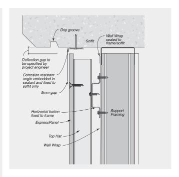
FIGURE 8.07 Base Detail - Drained
