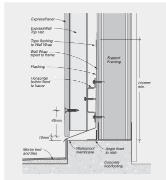
FIGURE 8.20 Typical Drain
