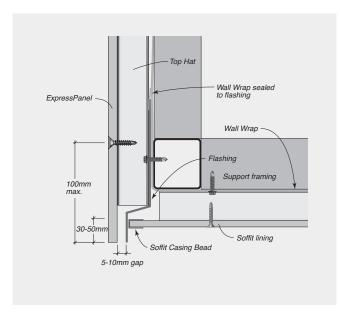
FIGURE 8.12 Control Joint - Vertical
