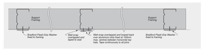
FIGURE 8.40 Vertical Wall Wrap Junction - Overlapped Single Strip Join
