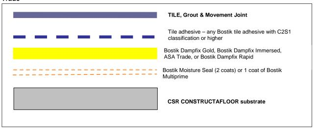
Variation 2 - Waterproofing using Dampfix PU
