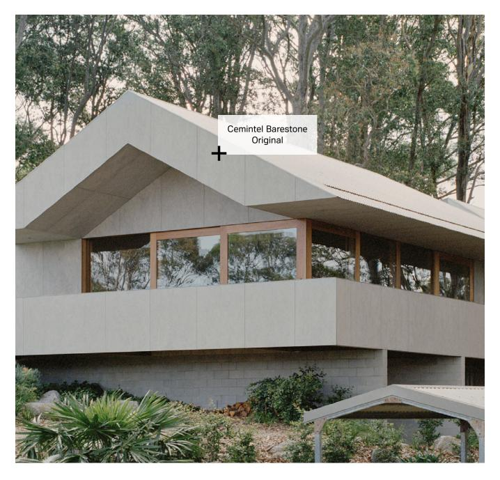
Barestone™ External can be used in many diverse ways and can be cut in many different shapes and sizes for dramatic design effect. The 9mm compressed panels incorporate Cemintel's unique CeminSeal® water block technology that repels water and they are manufactured in Australia.
